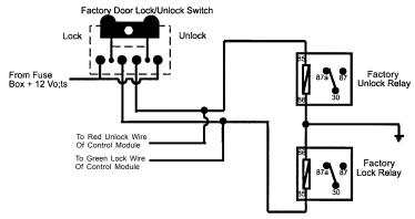
**NOTE:** For connection to Four Wire Polarity Reversal, 5 Wire Alternating 12 Volts, And All Other Door Lock Circuits the Audiovox AS-9159 Door Lock Interface, (or equivalent 30 A automotive relays) must be used. Refer to the Audiovox Door Lock Wiring Supplement for proper wiring of these circuits.
